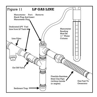
of the hard piping installation should include a sediment trap to drain any condensation and a line filter. (See Figure 11)
