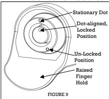
All generator access doors are locked, and are opened with a common key for all locks. Notice the door lock (in the locked position) has matching dot system i n alignment. Insert the key into lock
