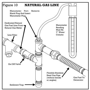
**NOTE:** After completion of all gas tests, remove manometer and replace blank plug, using fresh pipe sealant.
