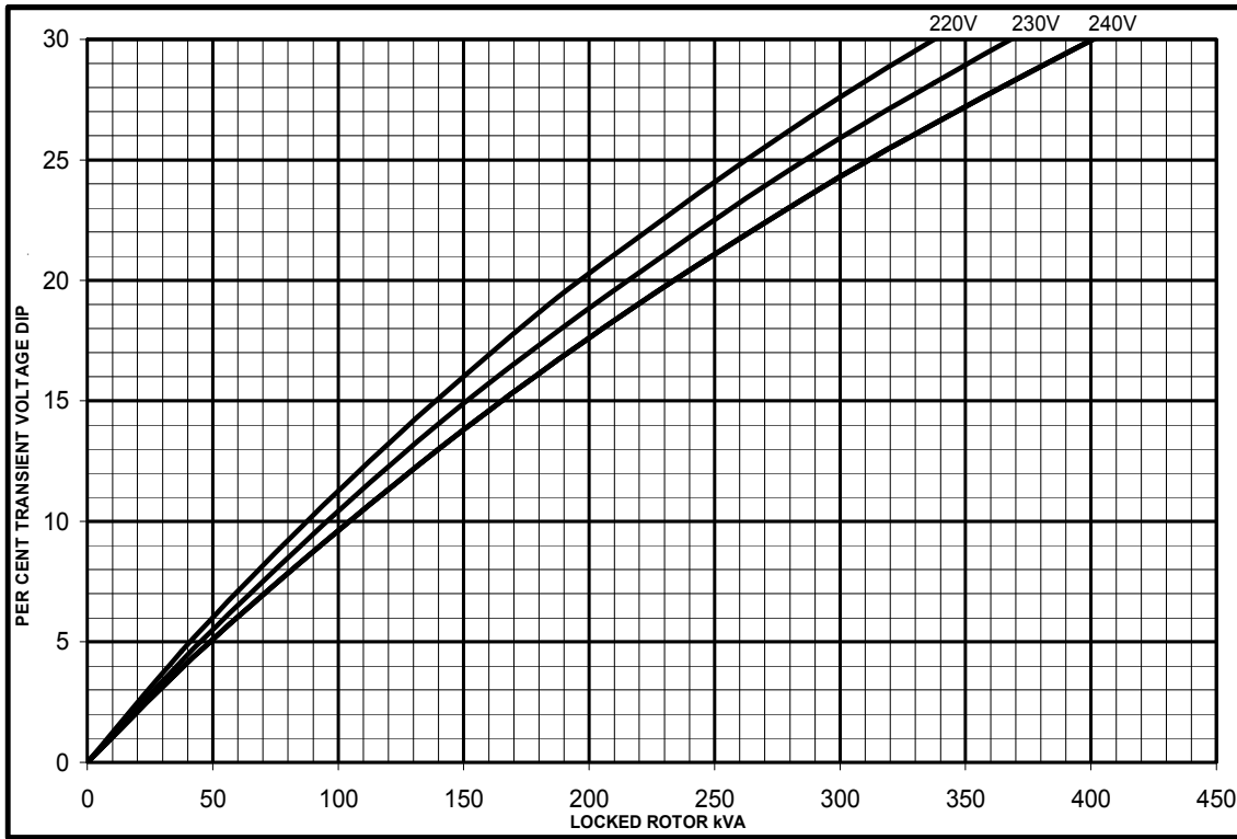
Locked Rotor Motor Starting Curves
