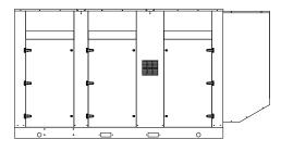
"LEVEL 2" HOUSED GEN-SET Full aluminum weather protection and superior sound attenuation for specific low noise applications. Critical grade muffler is standard.
